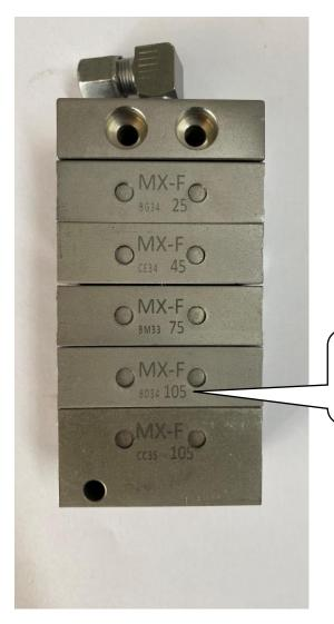
Beka blocks are bolted together. Each block can deliver different amounts of grease to each point.
