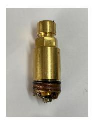
Twin system injectors come in sizes from 0 - 11 Refer to chart for grease capacity per cycle from each injector.
