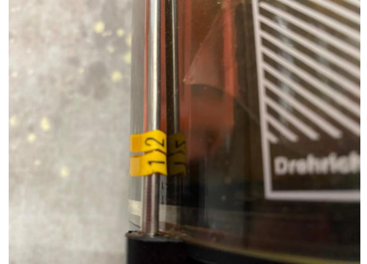
'12' Tag indicates 12 volts. No tag indicates 24 volts
