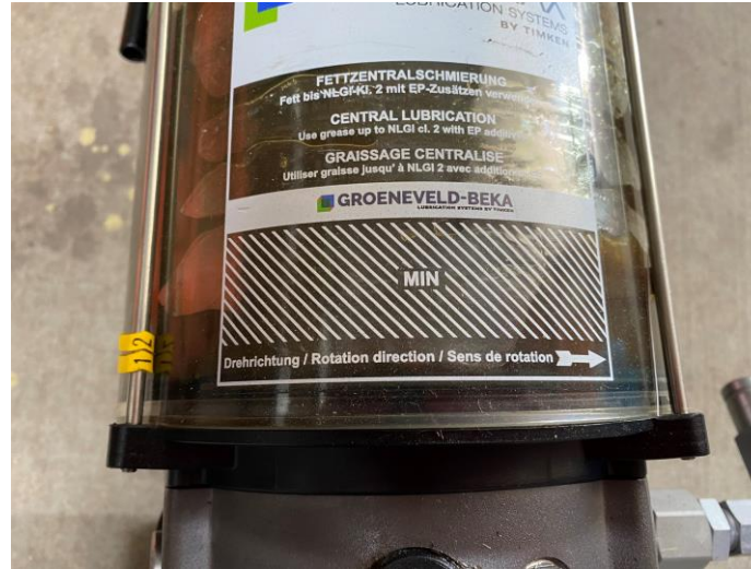
Pump voltage - 12 Volt has yellow tag, 24 Volt has no tag
