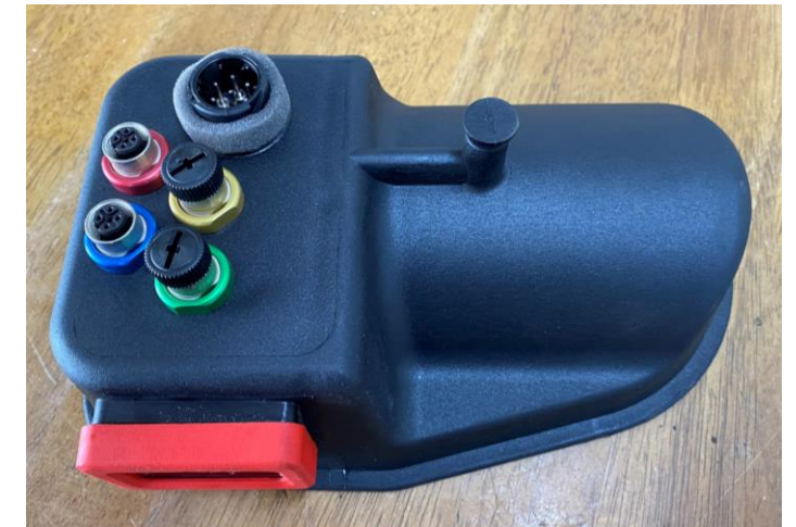
Low Level, High Pressure, Prox Switch, Error Indicator Controller (P10138124-R01)
